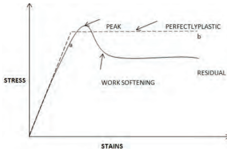
Figure 1(a): Elastic-perfectly plastic model (Kok Sien Ti et al., 2009)
