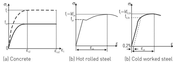
Figure 2: Stress strain curve for concrete and steel
