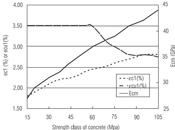
Figure 1: Change in modulus of elasticity and strain with grade of concrete
