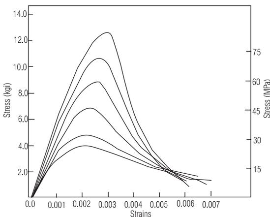
Figure 5: Stress-strain relationship of concrete with different strengths
