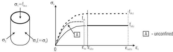
Figure 4: Stress strain relationship for concrete
