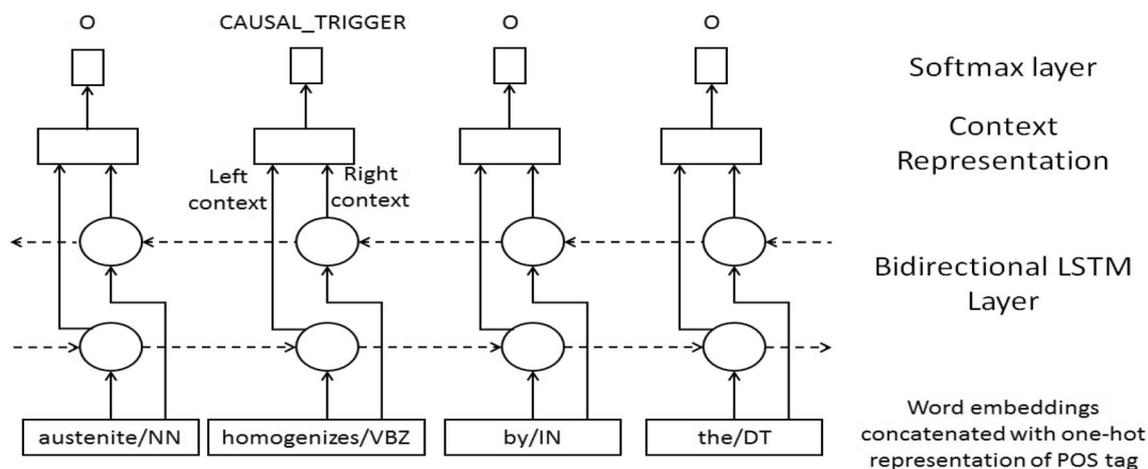
**Fig. 2** Bi-directional LSTM architecture for causal trigger detection
