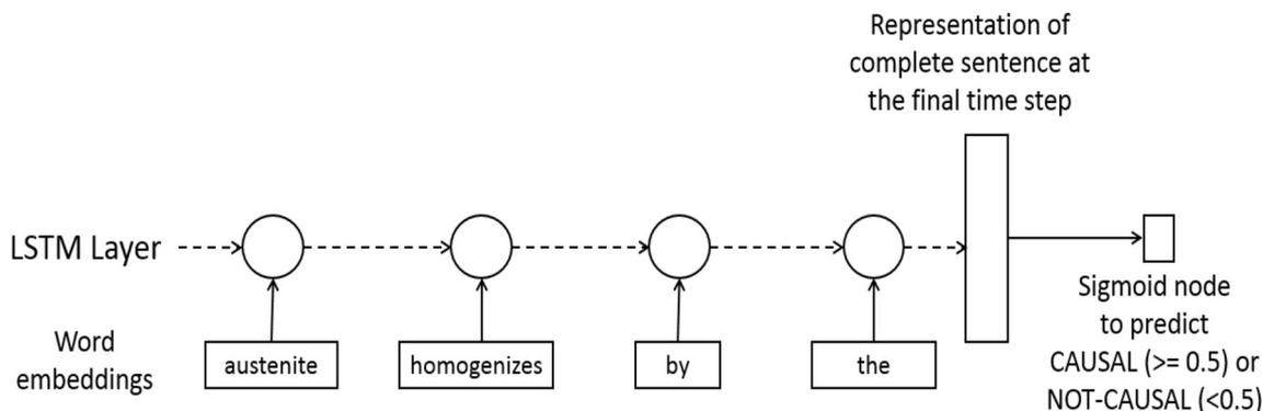
**Fig. 3** LSTM architecture for causal sentence identification
