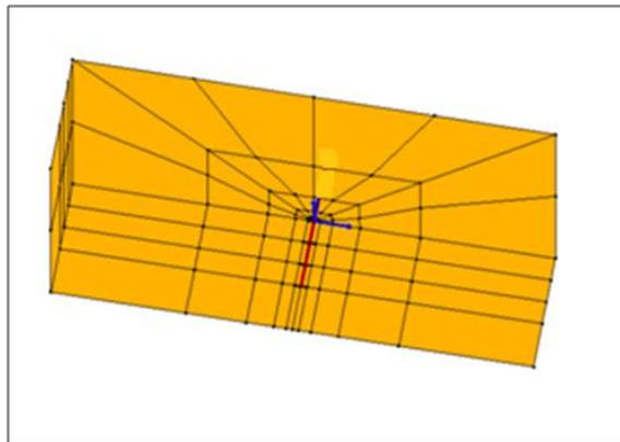
*Figure 1. Soil Pile Finite element model generated for study*
