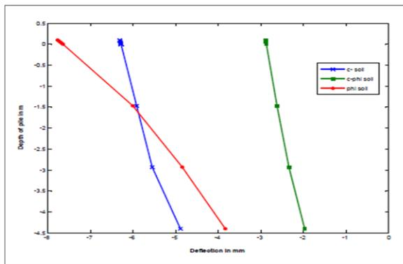
Figure 4. Deflection profile for short pile (L= 4.5 m) for different soil types
