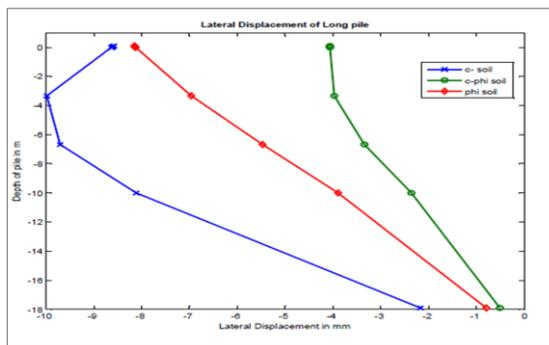
Figure 5. Deflection profile for long pile (L= 18 m) for different soil types
