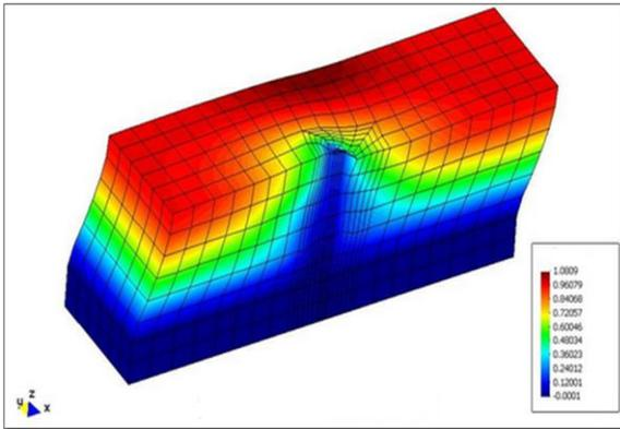
Figure 3. Stress contours in the soil strata after application of the dynamic loads
