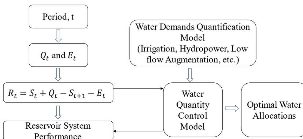
Figure 2. Water quantity control model of a reservoir.
