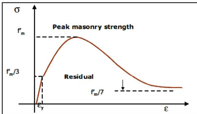
Fig. 5: Hardening and Softening Applied for Joint Spring in Compression Cap
