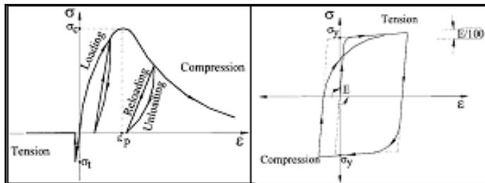
Fig. 6: Material Models for Concrete and Steel
