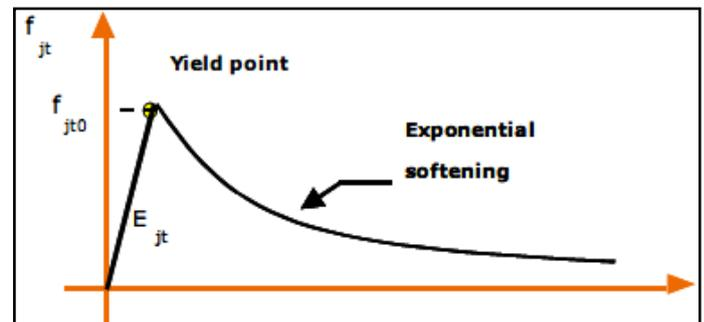
Fig. 3: Bond Degradation
