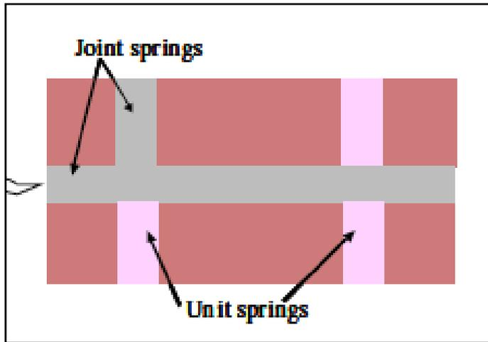
Fig. 1: Brick Masonry Discretization
