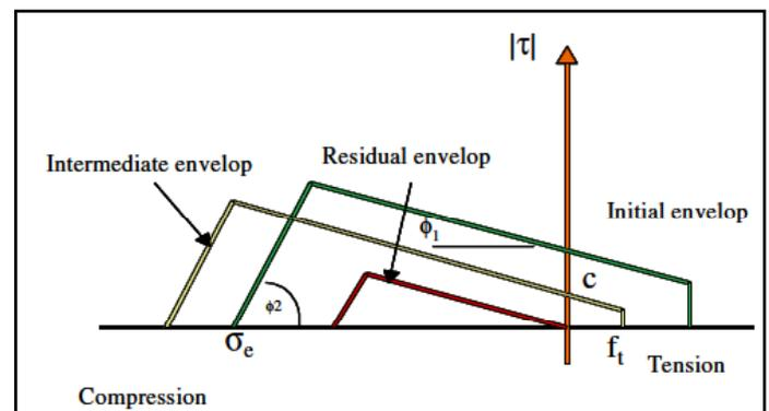
Fig. 4: Failure Criteria for Joint Spring
