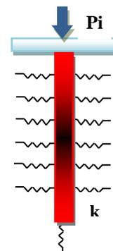
Fig. 2 Equivalent/single pile with soil represented as a spring for soil pile interaction analysis [25].
