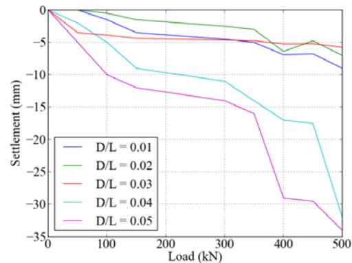
Fig.6b. Settlement for tank by EPM (empty condition).
