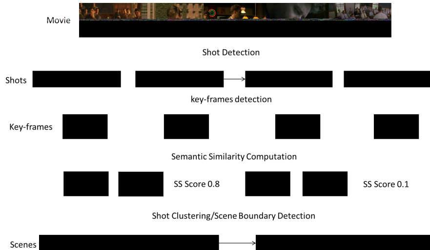
Fig. 1. This figure depicts a schematic flow of how the scenes are being detected in the movie. Initially we have the complete movie as input. We apply shot segmentation and key frame extraction to get the shots and key frames. Then Semantic Similarity Computation module computes semantic similarity between shots. The Semantic Similarity Score or SS Score has been shown in the figure for two pairs of shots. Then Scene Boundary detection module takes the shots and similarity score as input and output the scene boundaries.
