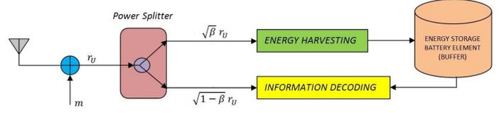
Fig. 2. Receiver architecture for power splitting (PS) scheme.
