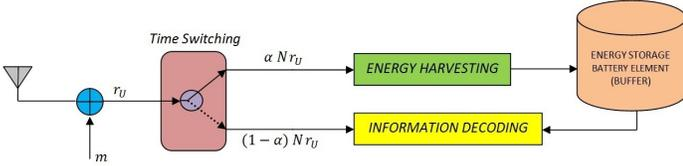
Fig. 1. Receiver architecture for time switching (TS) scheme.
