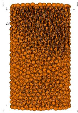
**Fig. 3** Triaxial specimen with velocity vectors
