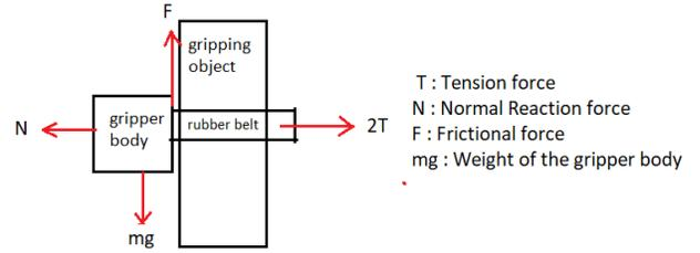
**Figure 7: Schematic diagram of gripper showing all the forces**
