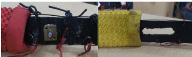
Figure 3: Rubber belts with locking motor and slit
