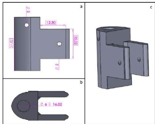
Figure 5: a) Front view of belt holder. b) Top view of belt holder. c) belt holder (all dimensions are in millimeters. Figure not to scale)
