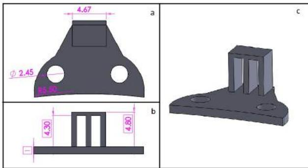
Figure 2: a) Top view of gripper base. b) Front view of gripper base. c) Gripper base (all dimensions are in centimeters. Figure not to scale)
