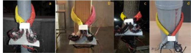
**Figure 9:** Gripping on a) Round metal pole (diameter : 80 mm) b) Square wooden pole (diagonal : 137.8 mm) c) Tree (diameter : 117.8 mm) d) Circular PVC pipe (diameter : 165.6 mm)
