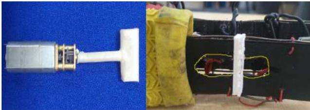
**Figure 8:** a) Motor with T-shaped shaft for locking b) After locking together both belts (yellow line shows slit through which the shaft passed)
