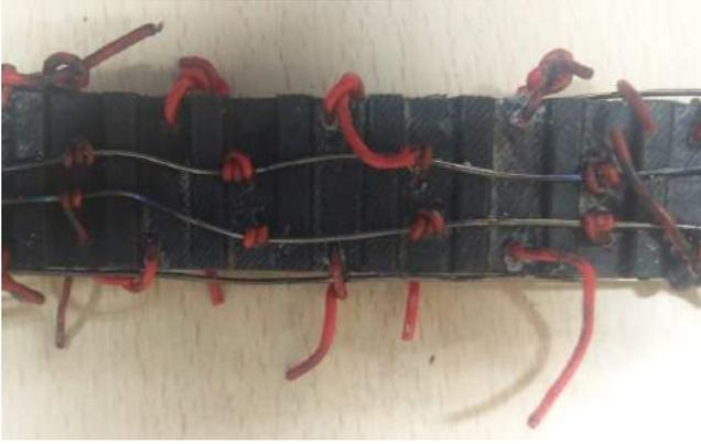
**Figure 6: SMA fastened on rubber belt using high temperature grade silicone wire**
