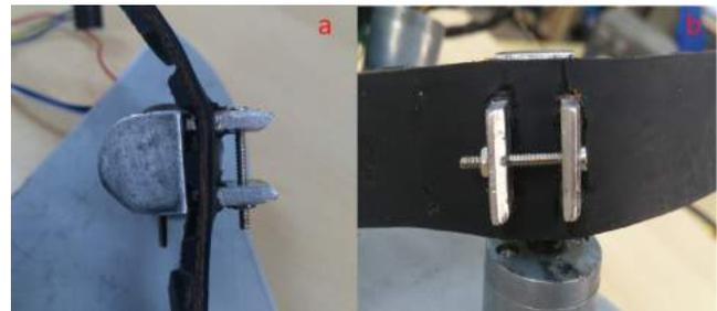
Figure 4: Rubber belts attached on belt holders in a) Top view b) Front view
