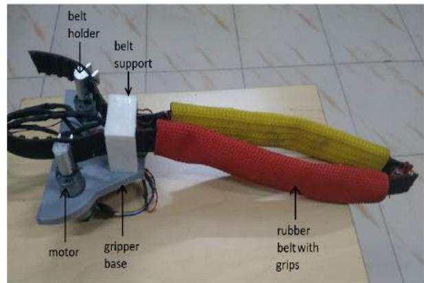
Figure 1: Prototype of flexible gripper.
