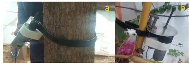
**Figure 10:** Gripping on a) thick tree trunk (diameter : 120 mm) b) Bamboo stem (diameter : 25 mm)
