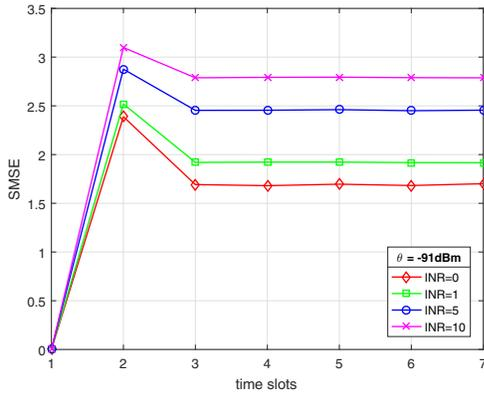
Fig. 4: Variation of SMSE over time, for different values of INR, at  $\theta = -91\text{dBm}$  and SNR = 10dB.
