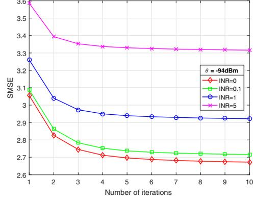
Fig. 3: Number of iterations required to obtain optimal  $\mathbf{F}, \mathbf{V}$ , for different values of INR, for  $\theta = -94\text{dBm}$  and  $\text{SNR} = 5\text{dB}$ .
