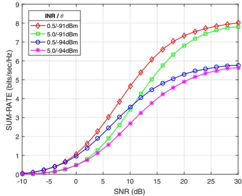
Fig. 6: Sum-rate, in the 7<sup>th</sup> time slot, versus SNR, for different values of INR and  $\theta$ .
