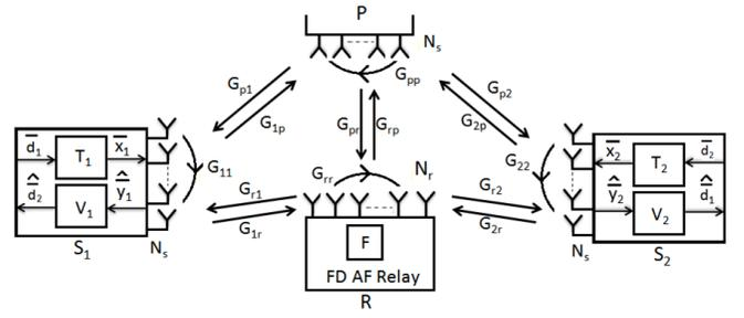
Fig. 1: System diagram of a FD two-way cognitive radio network.
