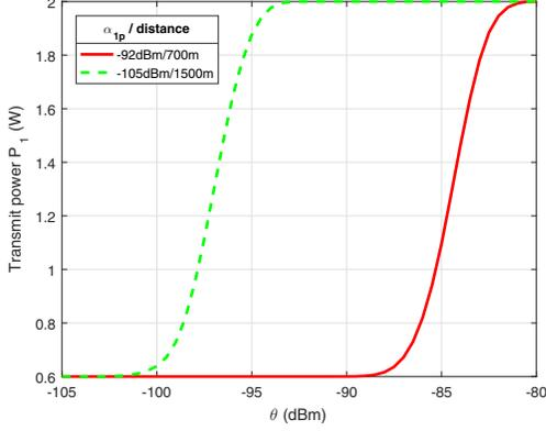
Fig. 2: Variation of transmit power versus  $\theta$ , for different values of path loss.
