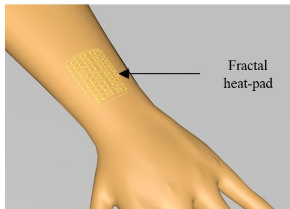
Fig. 1. Illustration of a flexible metallic heat-pad based on a fractal metal coil design.
