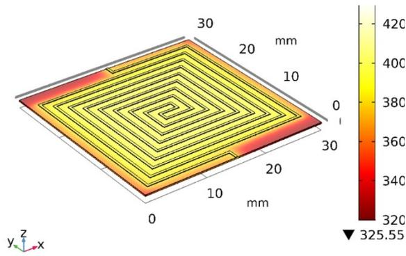
Fig. 8. 3D surface temperature plot of a double spiral heat-pad with 1 W input power.
