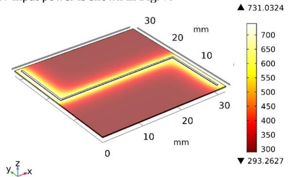
Fig. 7. 3D surface temperature plot of wire-line heat-pad for 1 W input power.
