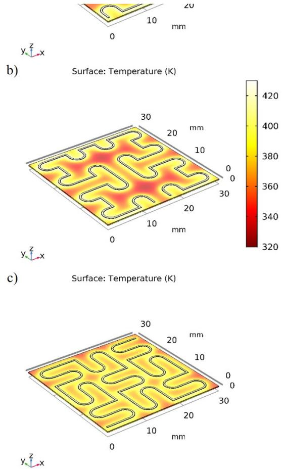
Fig. 9. 3D surface temperature plots of (a) Hilbert order-3 (b) Moore order-3 and (c) Peano order-2 curves. Color legend for all the temperature plots is common.
