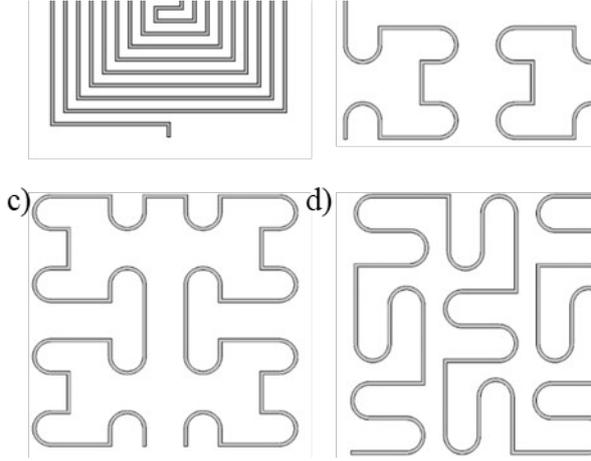
Fig. 5. Simulated metal coil geometries based on (a) double spiral, (b) Hilbert order-3, (c) Moore order-3 and (d) Peano order-2 curves.
