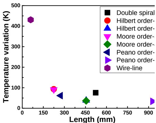
Fig. 12. Plot of temperature variance versus the length of a metal coil for 1 W input power.
