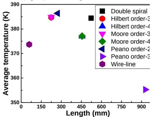
Fig. 11. Plot of average temperature versus length of a metal coil for 1 W input power.
