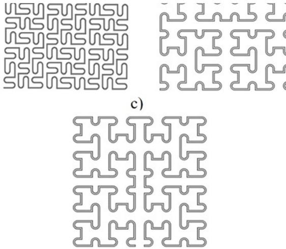
Fig. 6. Simulated metal coil geometries based on (a) Peano order-3, (b) Hilbert order-4 and (c) Moore order-4 curves.
