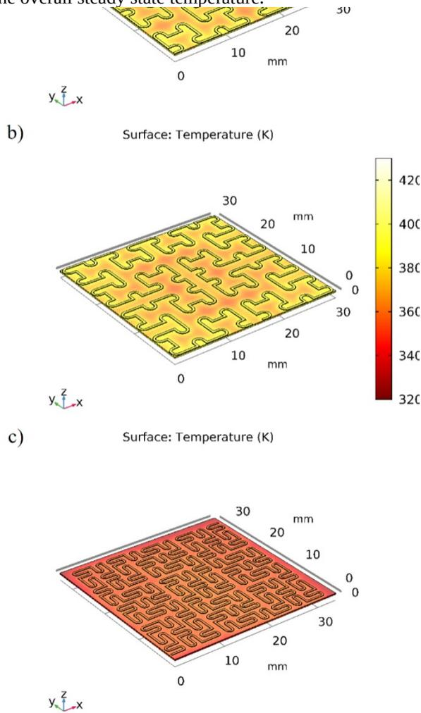
Fig. 10. 3D surface temperature plots of (a) Hilbert order-4 (b) Moore order-4 (c) Peano order-3 curves. Color legend for all the temperature plots is common.
