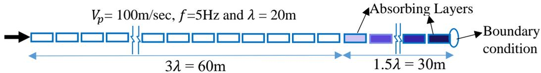
**Figure 1:** Configuration for one dimensional wave propagation model
