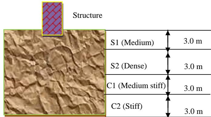
Figure 2. Details of soil layers considered in present study.
