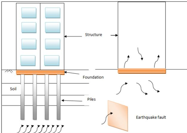
Figure 1. General scenario of consideration of soil structure interaction effect and wave propagation [13].
