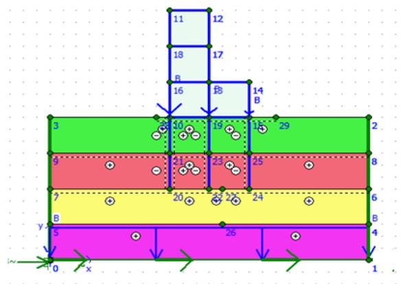
Figure 4. Finite Element model for the interaction analysis.
