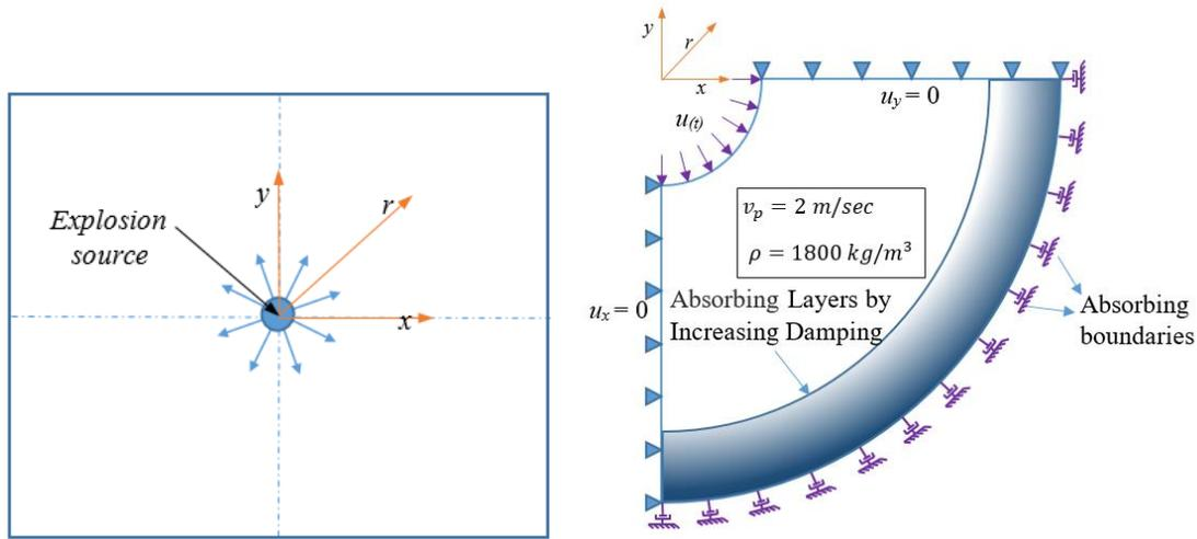
**Figure 1.** 2D Plane strain model for pure P-Wave propagation
