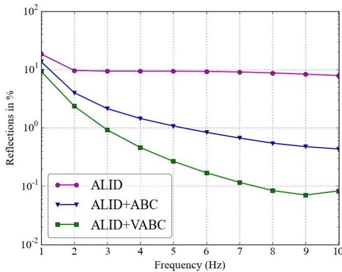
**Figure 2:** Percentage of reflection for three different configurations against design load frequency
