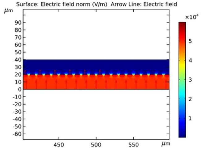
Fig. 6. Finite element analysis (FEA) simulation of a two-layer capacitance system, with bottom electrode at high voltage and top and middle electrode at ground.
