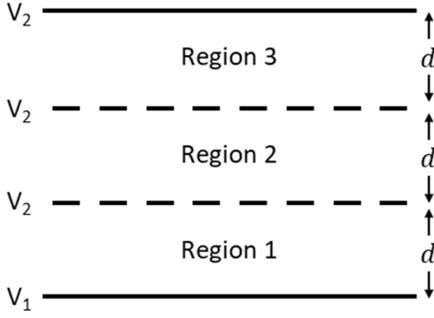
Fig. 4. Schematic illustration for a three-layer capacitance system with two perforated electrodes.
