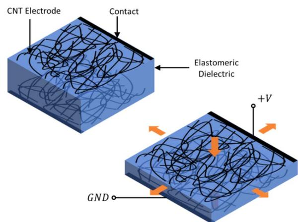
Fig. 1. Schematic illustration of a single layer dielectric elastomer actuator using CNT-based electrodes.
