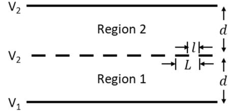
Fig. 3. Schematic illustration of a two-layer capacitance system with perforated central electrode.
