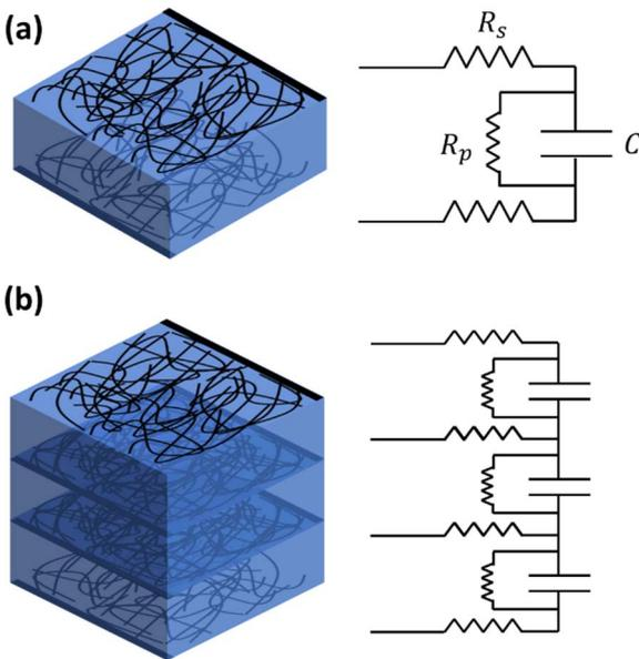
Fig. 2. Capacitor/resistor model for (a) single layer DEA, (b) multilayer DEA.
