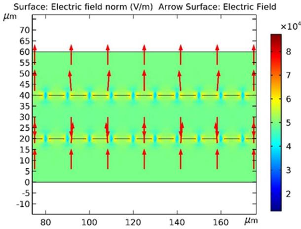
Fig. 7. Finite element analysis (FEA) simulation of a three-layer capacitance system, with alternate electrodes at high voltage and ground. The arrows indicate the direction of the electric field.
