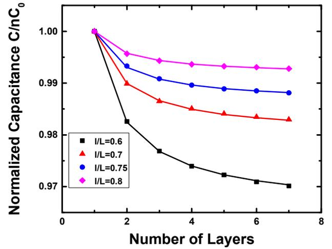
Fig. 8. Normalized capacitance versus number of layers for an interdigitated multilayer capacitance system with perforated intermediate electrodes. The dots represent simulated capacitance values from FEA, while the lines represent capacitance values calculated from theory.
