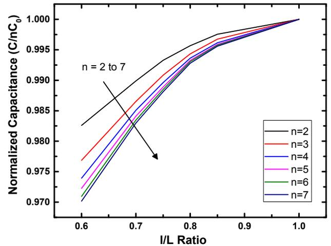
Fig. 9. Variation of normalized capacitance with perforation ratio ( $l/L$ ) for different number of layers.
