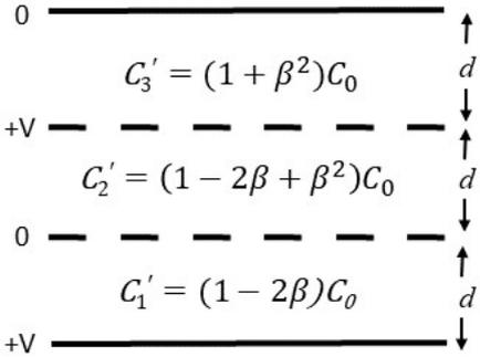
Fig. 5. A three-layer capacitance system with two perforated electrodes with alternate high voltage and ground connections.
