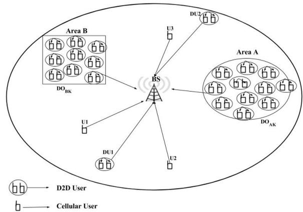
Fig. 1: System model for multiple D2D connections in a cell illustrating interference between D2D users in Area A and Area B
