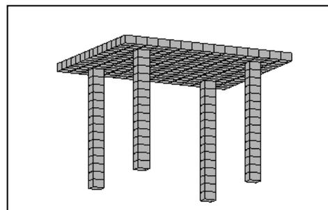
Figure 5: 3D Model of flat slab structure
