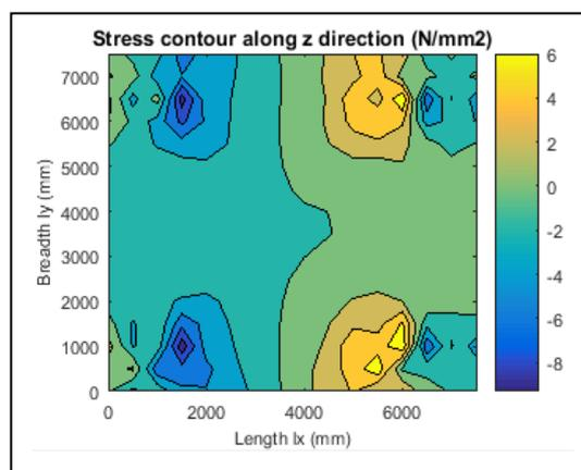
Figure 9: Stress concentration on the slab
