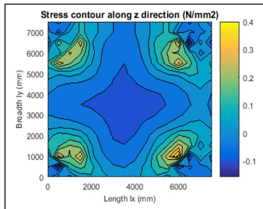
Figure 7: Stress concentration on the slab
