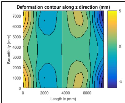
Figure 10: Top deflection of slab
