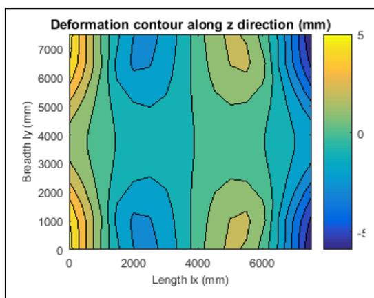
Figure 8: Top deflection of slab
