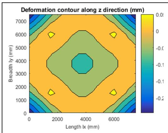
Figure 6: Top deflection of slab
