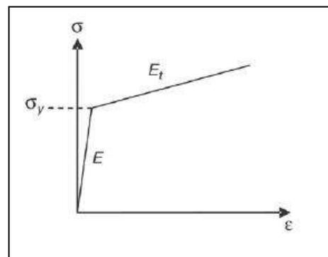
Figure 3: Bilinear model of concrete
