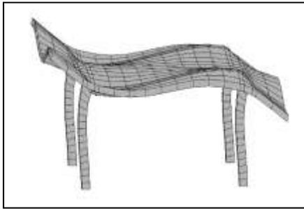
Figure 1: Punching shear of slab around column
