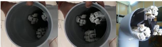
**Figure 10: Modular Pipe Climber Negotiating a Turn in a  $90^\circ$  Bend.**
