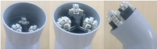
**Figure 9: Modular Pipe Climber Negotiating a Turn in a  $45^\circ$  Bend.**
