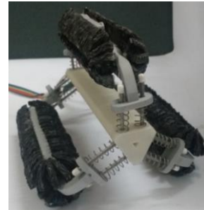
Fig.1: Omnidirectional Tractable Three Module Robot.
