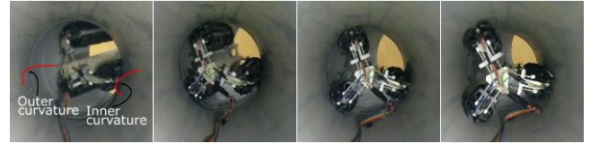
Fig.15: Robot traversing in an elbow with the preferred orientation where one module takes the innermost curvature.
