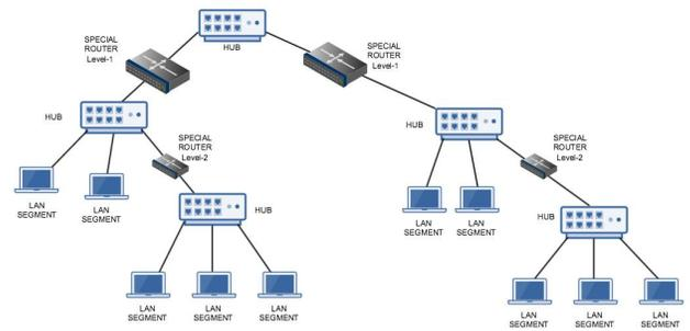
Fig. 1. Distributed Backbone Network
