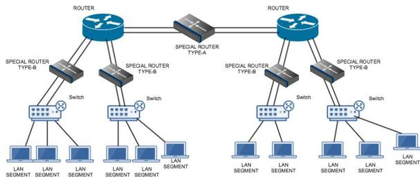
Fig. 3. Parallel Backbone Network
