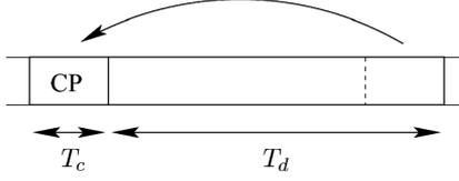
Figure 2. A cyclic prefix of  $T_c$  symbols is copied in front of the data block of  $T_d$  symbols to create one OFDM symbol or block containing total  $T_s = T_d + T_c$  symbols.
