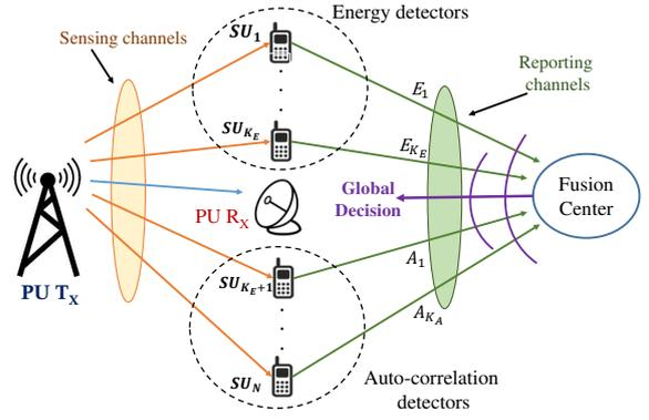
Figure 1. System model for the considered heterogeneous CSS using  $K_E$  number of energy detectors (EDs) and  $K_A$  number of autocorrelation detectors (ADs).
