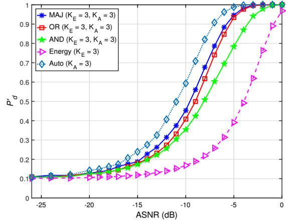
Figure 5.  $P_d$  vs SNR (dB) plot showing comparison of soft and hard combining schemes in the presence of noise uncertainty with  $\sigma_\Delta^2 = 0.1$  and average  $P'_{f,fc} = 0.1$
