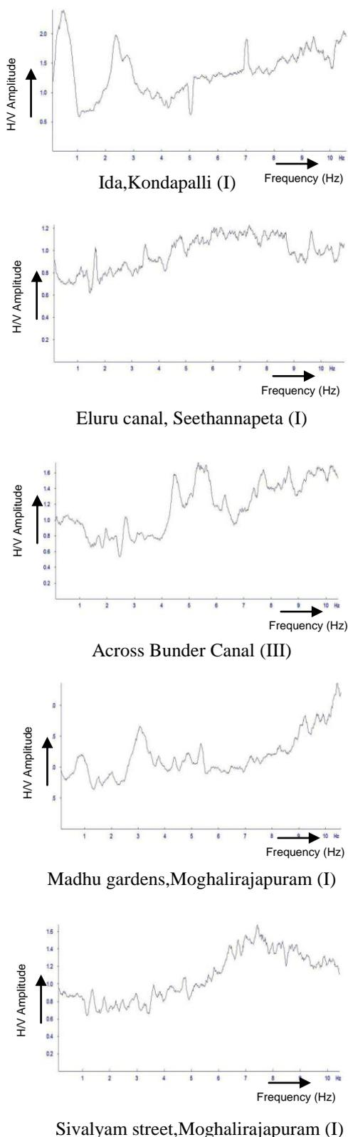
**Fig. 2** H/V Amplitude vs. Predominant frequency curves at different test sites
