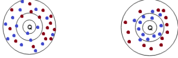
Figure 2. Toy image showcasing the distribution of the samples before and after the fine tuning using triplet loss. The red/blue dots indicate negative/positive examples. The innermost circle resembles the boundary for the Query image. The outermost circle is imaginary resembling the maximum distance a sample image can be from the query. The middle circle is indicative of the margin which we use to separate the positive samples from the negative samples.
