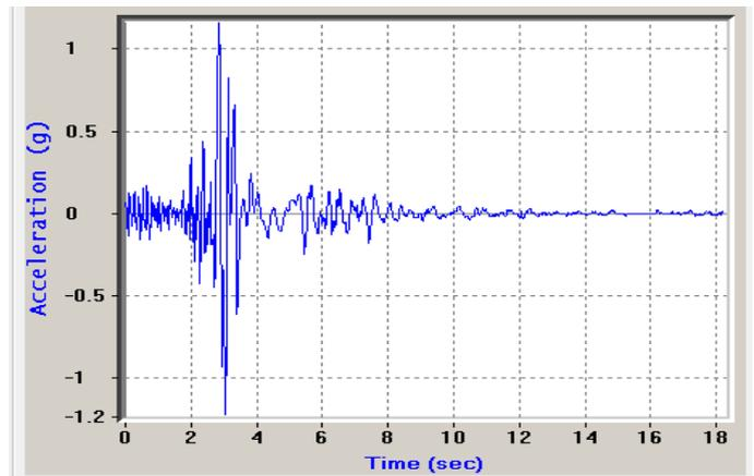
Fig 1. Acceleration time history of 1995 Chamba Earthquake
