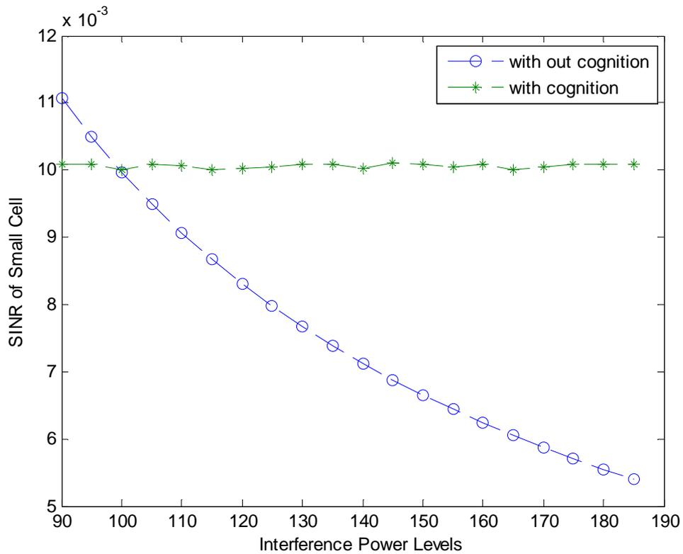
Figure 10. Comparison of SINR of small cell with and without employing cognition
