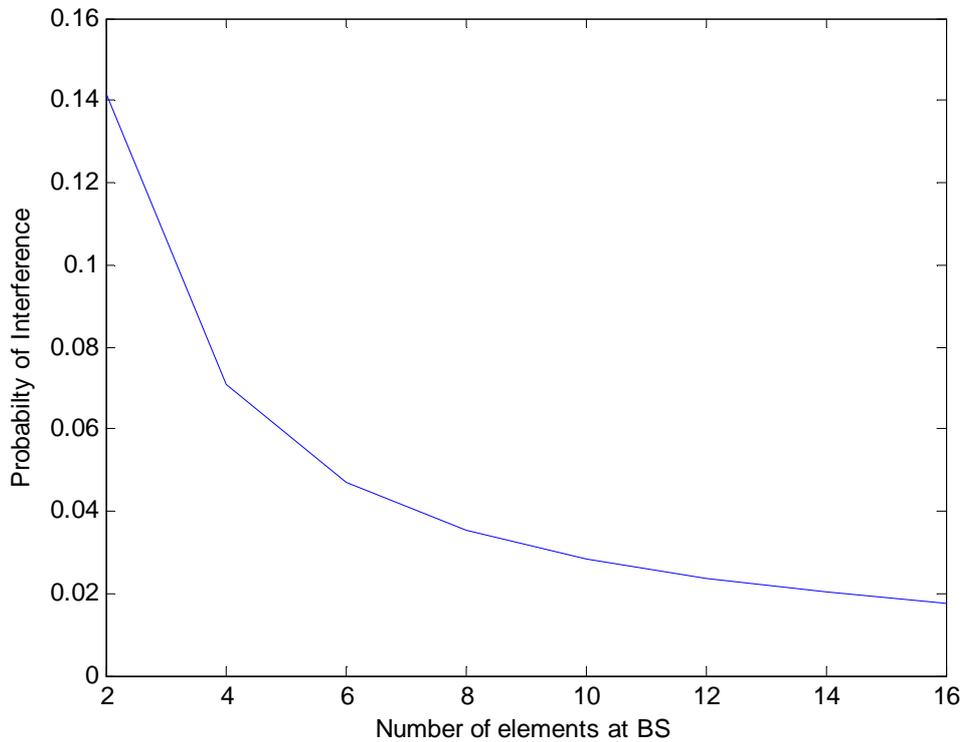
**Figure 15. Number of antenna elements at femto cell access point vs probability of interference to nearby macro users**
