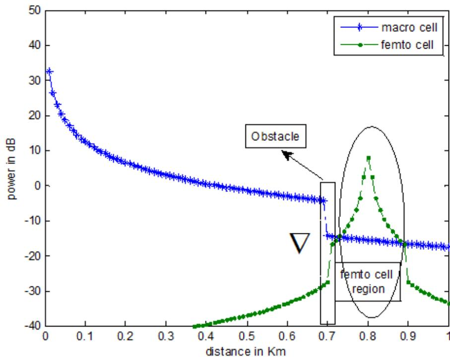
**Figure 8. Macro cell and Femto cell Power levels vs Distance**
