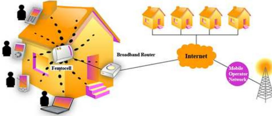
**Figure 7. Femto cell connection to mobile operator [14]**
