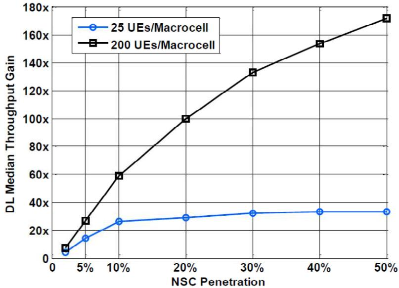
Figure 2: DL user throughput gains for a (10 + 10) MHz NSC deployment relative to 10 MHz macro carrier baseline for 25 or 200 active users per macrocell area [5].
