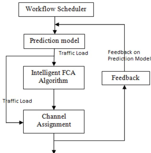
Figure 3: Work flow - Optimal Hybrid Channel Allocation
