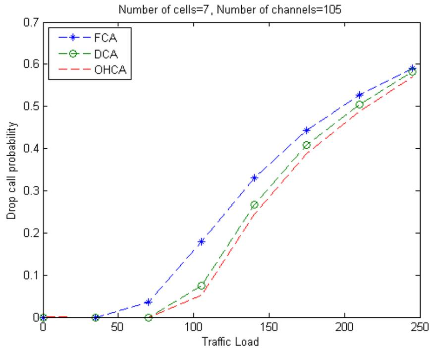
**Figure 5: Drop call probability vs Traffic load**
