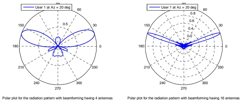
**Figure 12. Polar plot of Radiation Pattern with beam forming having 4 and 16 antennas**
