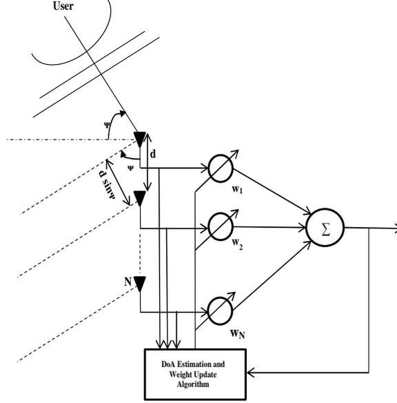
**Figure 13: Adaptive Beam former Architecture using uniform linear antenna array with  $N$  elements and inter element distance ' $d$ '**
