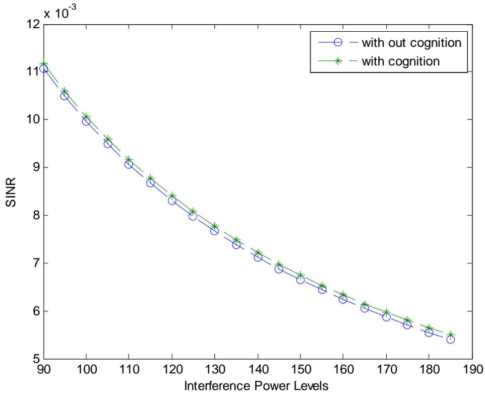
Figure 11. Effect of cognition on SINR of neighboring Small cell
