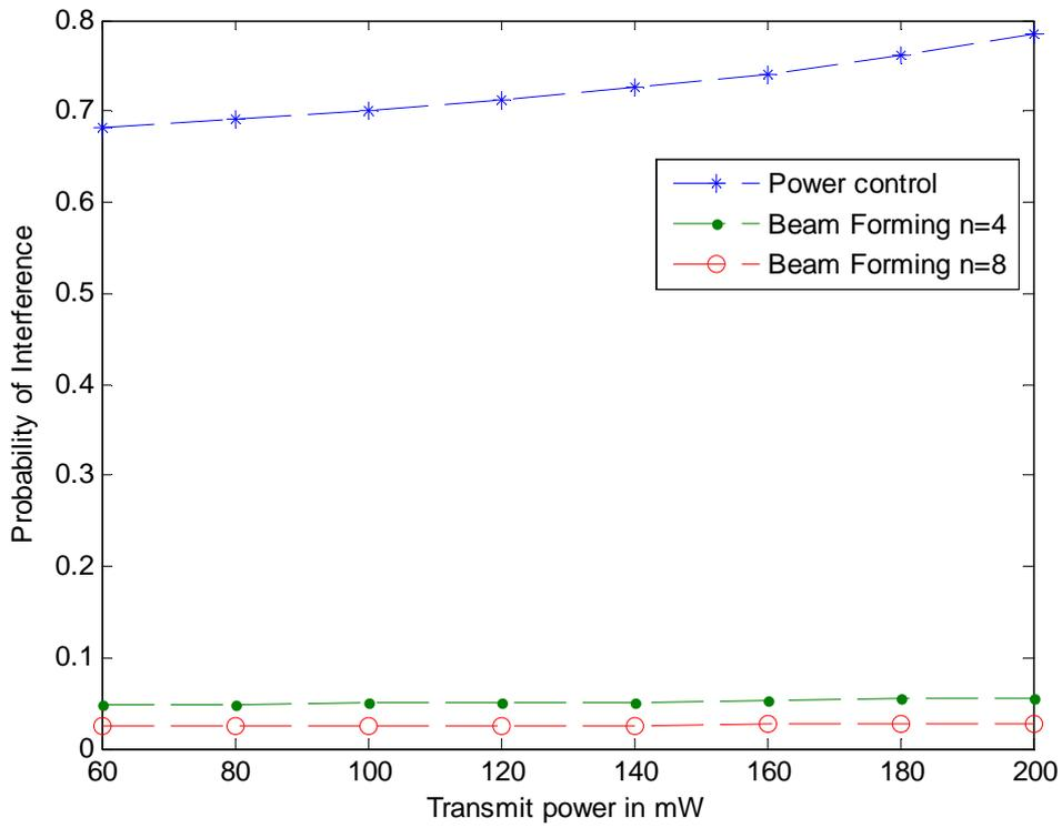
**Figure 14: Femto cell access point transmit power vs probability of interference to nearby macro users**
