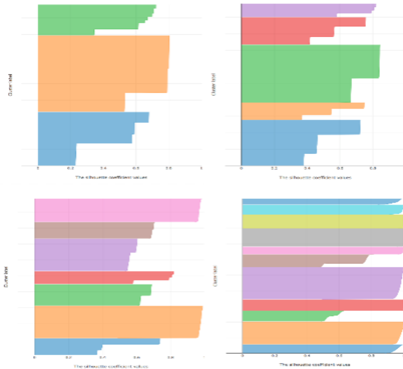
Figure 5.4 This figure has four silhouette plots with x-axis: silhouette coefficient value and y-axis: different colour corresponding to different cluster label. In each plot the value of k is varied. Top left K=3 , top right K=5 , bottom left K=7 , bottom right K=11 . We see that with increasing K value the clusters become lot more uniform with less fluctuations.
