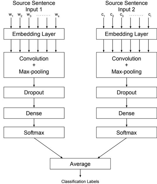
Figure 4: multiInput-CNN architecture as proposed by Tummalapalli et al. (2018)
