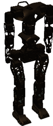
Figure 1 27 DoF humanoid robot with articulated torso.
